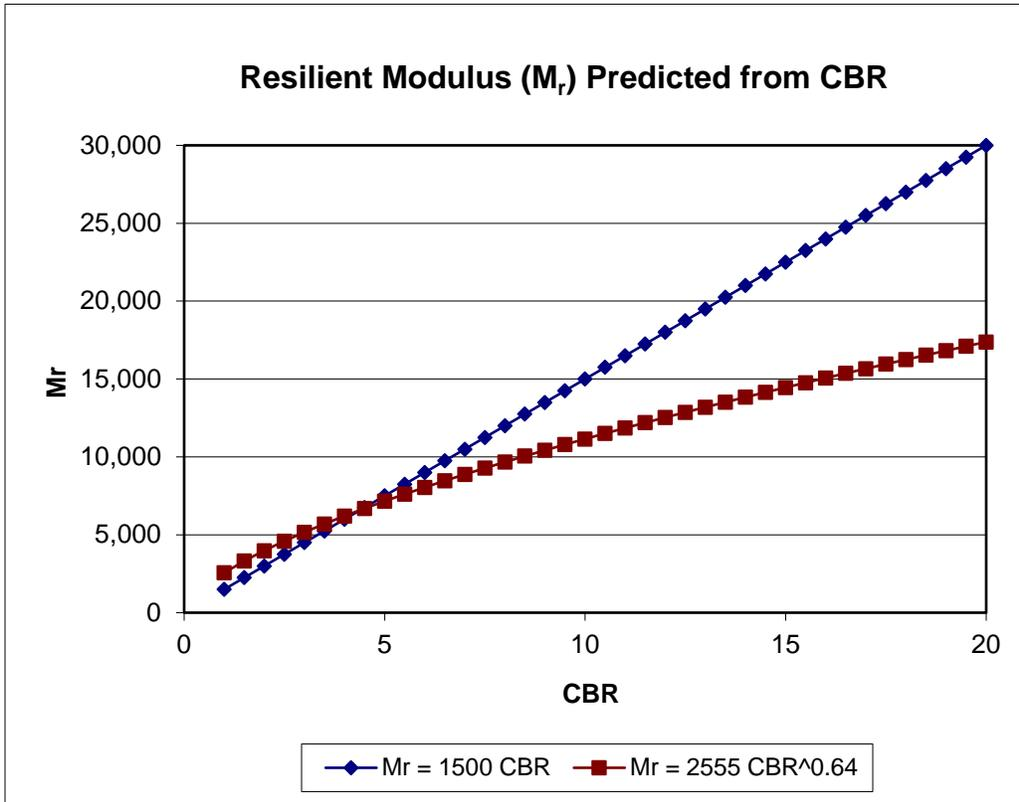
Figure 1. Resilient Modulus ( $M_r$ ) of Subgrade or Base as a Function of California Bearing Ratio (CBR) Using AASHTO 1993 and ME Models.
