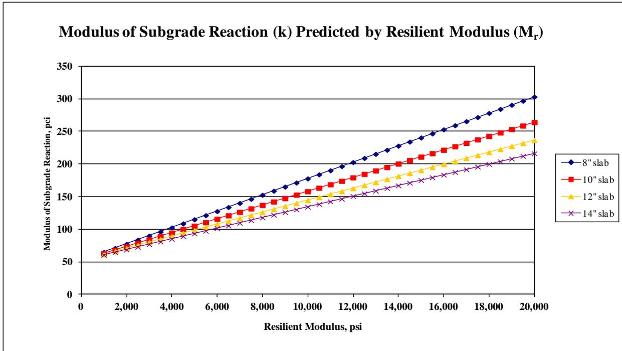
Figure 2. Modulus of Subgrade Reaction (k) of Subgrade or Base as a Function of Resilient Modulus ( $M_r$ ) Utilizing Equivalent Deflection Analysis.
