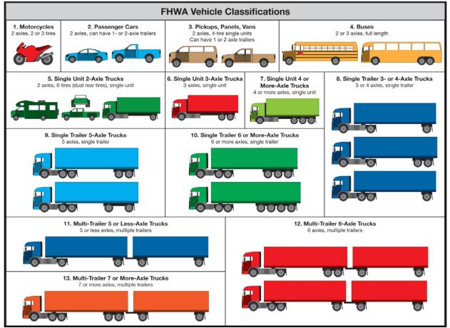
Figure 1. Graphical Reference to FHWA Vehicle Classifications. (Source: TxDOT Traffic Recorder Instruction Manual, February 2012, Copyright © 2012 by Texas Department of Transportation)
