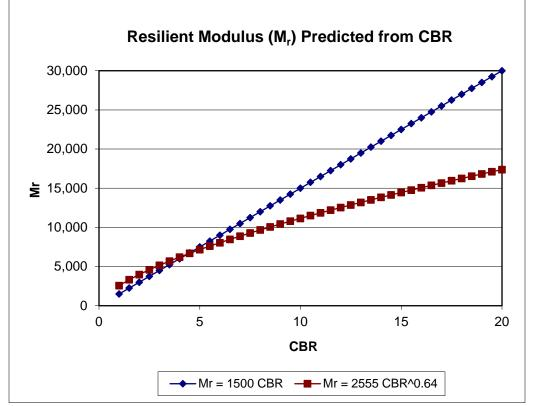
Figure 1. Resilient Modulus (M<sub>r</sub>) of Subgrade or Base as a Function of California Bearing Ratio (CBR) Using AASHTO 1993 and ME Models.
