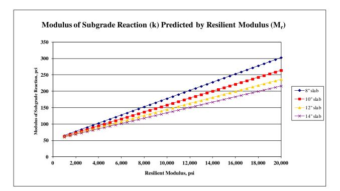
Figure 2. Modulus of Subgrade Reaction (k) of Subgrade or Base as a Function of Resilient Modulus (M<sub>r</sub>) Utilizing Equivalent Deflection Analysis.
