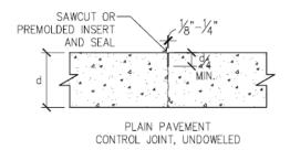
If the full width of pavement is paved together, longitudinal joints shall be sawcut to a minimum depth of 1/4 the concrete slab thickness and sealed with no tie bars required. If each pavement lane is paved independently the pavement lanes may be tied with 24 inch long 5/8 inch diameter Grade 60 deformed steel bars placed on 30 inch centers. Local experience may indicate that tie bars are not required with the confinement provided by the curb and gutter.
